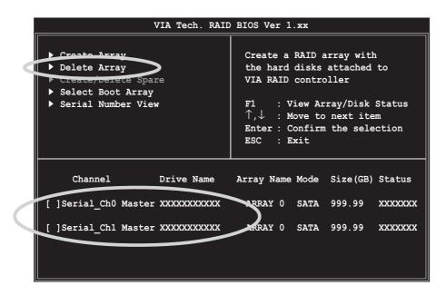
2. From the list of channel used for IDE RAID arrays, press **<Enter>** to select a RAID array to delete. The following confirmation message appears.
